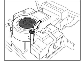
The oil level should lie between the markings on dip stick. If the level approaches the "ADD" mark, top up with oil to the "FULL" mark.
